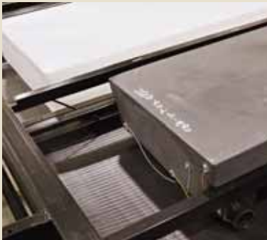
Heated and enclosed holding tanks (60 gallon fresh!) along with ducted floor heat, and solid steel I beam frame are first class!
