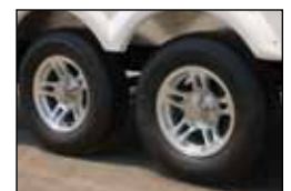
Cast aluminum wheels with radial tires
