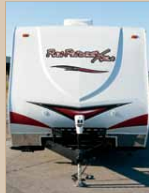
Front fiberglass cap with graphics, removable front storage tray and diamond plate rockguard.
