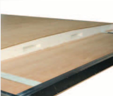
Vacuum-bonded roof with 2" radius
