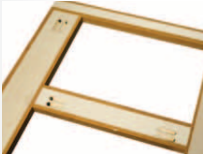
Glued and screwed wood cabinetry
